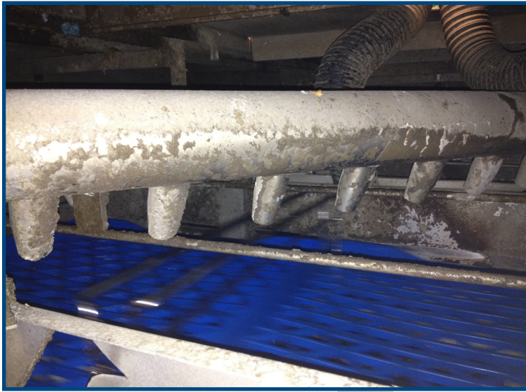
Blue plastic trays are dried by Paxton nozzle manifold
