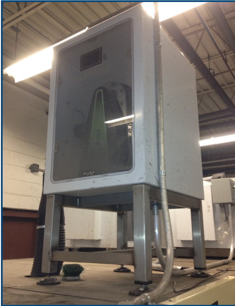
XT-500 blower powers two cone manifolds drying the tray bottoms
