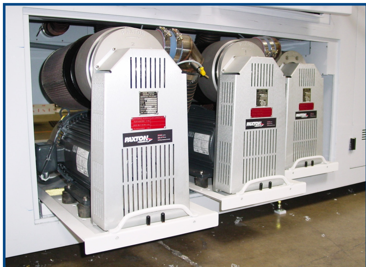
Each Nu/Clean has three Paxton AT-Series blowers
