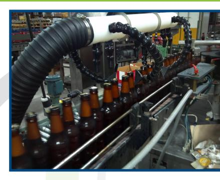
was positioned above the single line conveyor, just before the bottles enter the labeling machine. It takes up almost no space at all—which is pretty impressive considering how effective it is. We used to
